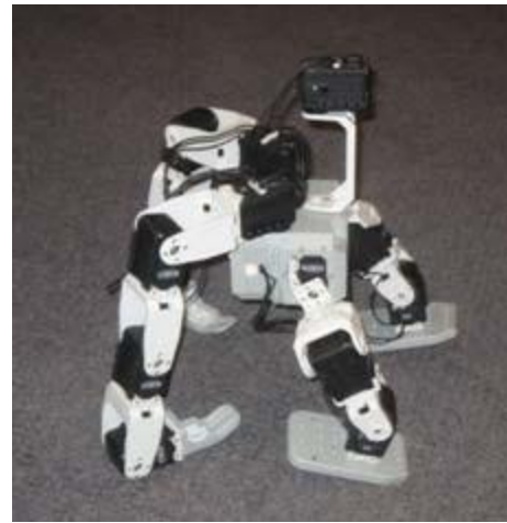
Figure 6: Ape-like robot, designed to perform knuckle-walking and allow a bipedal stance.
