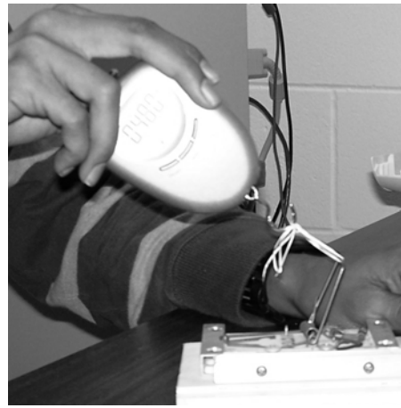
Figure 4. Twisting the mousetrap spring experiment.
