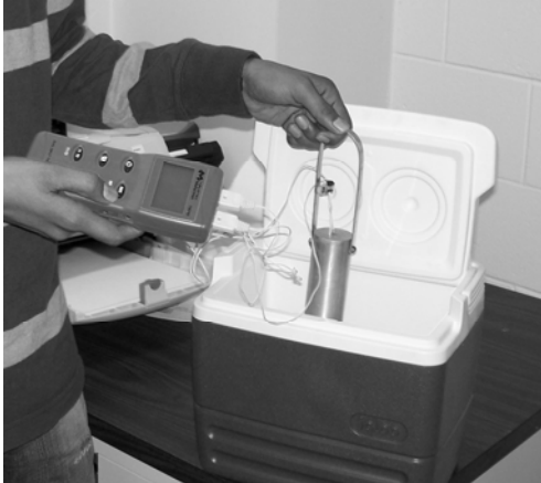
Figure 1. Immersing aluminum cylinder in iced-water experiment.
