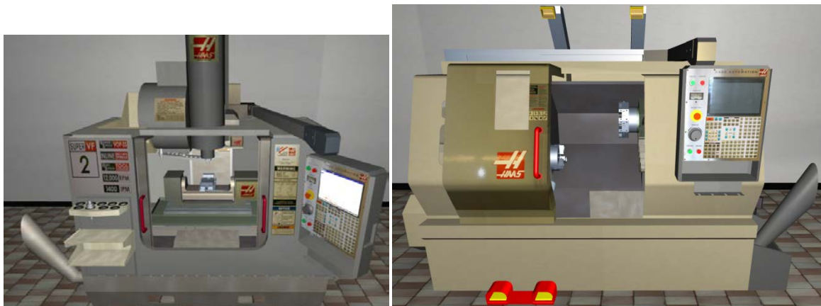
Figure 11. Interactive model of a HAAS Super VF-2 5-axis milling machine (left), and a HAAS SL-20 turning machine (right).
