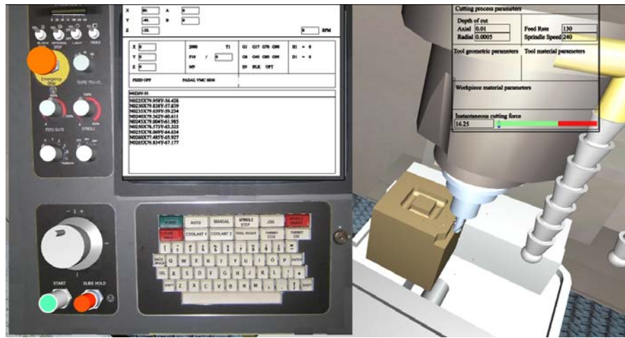
Figure 12. Virtual machining of a work piece on a 3-axis milling machine. The machine controller View, on the left, shows the current NC-code line that is being executed. The machining monitor, on the top right, shows the machining parameters and estimated values of the cutting forces.
