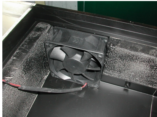
Figure 5: The outlet fan.
