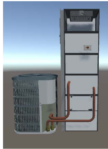
Fig. 5. 3D model of HVAC System
