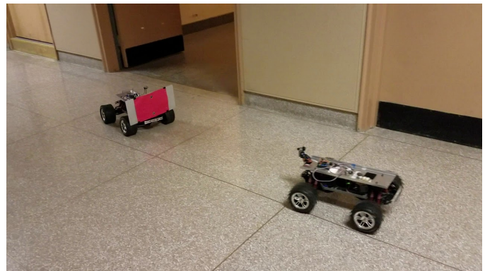
Fig. 3. Picture showing a pair of leader-follower robots in the hallway of our academic building. The camera mounted on the front of the follower vehicle is visible. The red paper on the leader is an easy-to-find target for computer vision.
