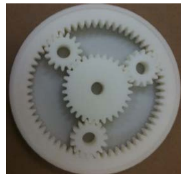
Figure 10. 3D printing result for gear train example.
