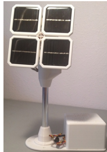
Figure 18. Photovoltaic Tracking System.
