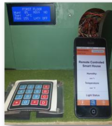
Figure 1(c). Local and Remote Control of the House
