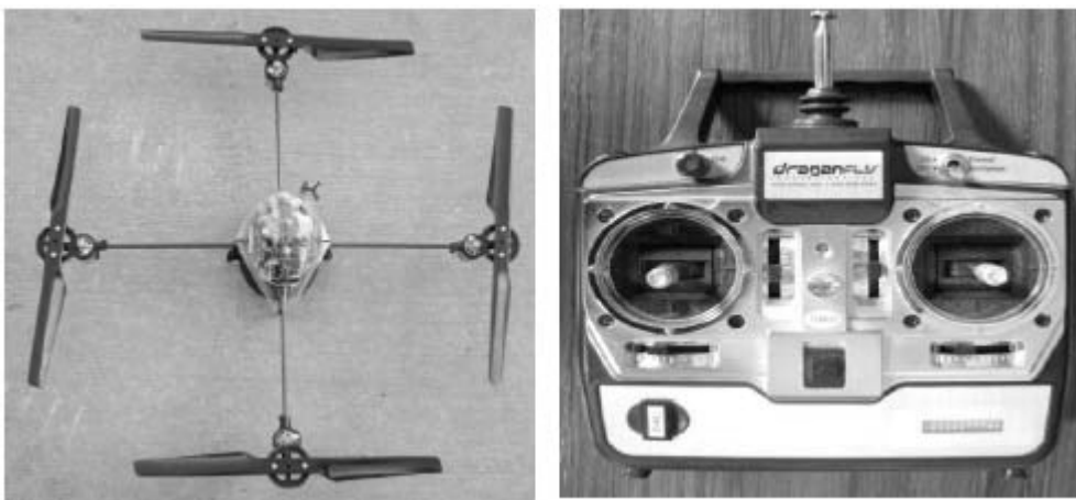
Figure 2. The Draganflyer quad-rotor and transmitter.
